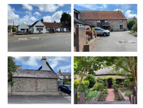
Fig 18: Various roof materials: thatch, clay tiles, slate, Horsham slab
